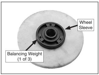
Figure 31. Weights evenly distributed around wheel sleeve groove.
